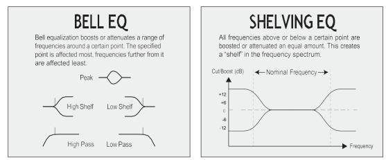
Next, you'll have bell-shaped low-mid and high-mid bands with fully adjustable gain, frequency and Q (bandwidth) parameters.
